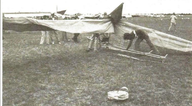
Opening up the wings. The entire machine is wire braced — using aircraft cable.
