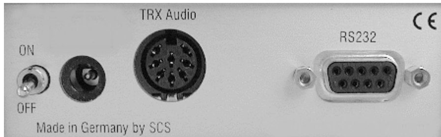
Figure 3.1: The PTC-IIe rear panel.
